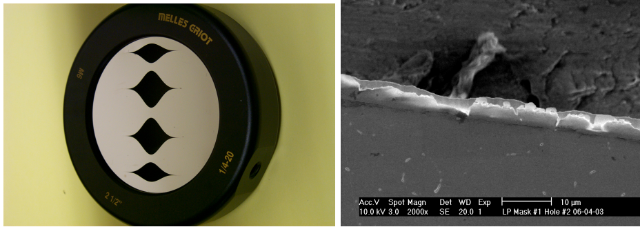
Figure 10. Left A four pupil mask made from Nickel via electroforming. Right An SEM image of the edge of the mask.
