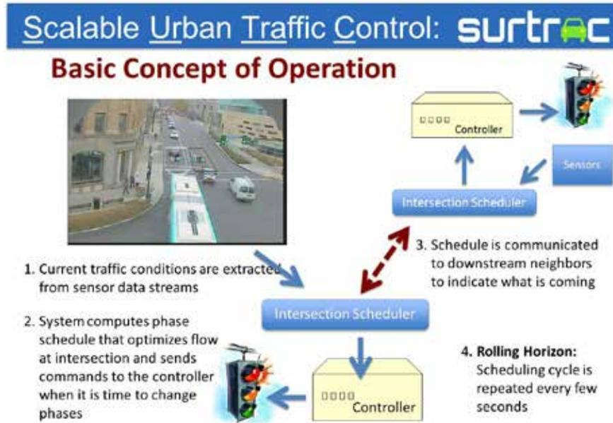
**FIGURE 3 Scalable urban traffic control system concept of operation.**
