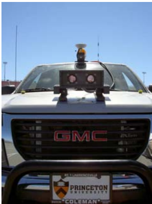
Figure 2.1 Prospect Eleven's Stereo camera and GPS boom
