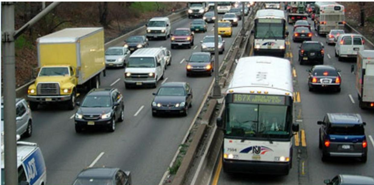
**FIGURE 1 Exclusive Bus Lane (XBL) Contra-Flow Bus Lane in Operation**
